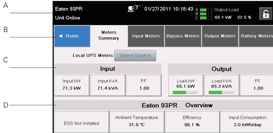
**Figure 6-2: Parts of the Display**
